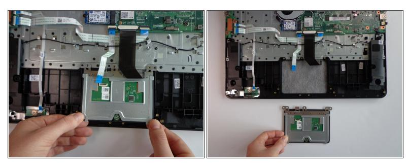
Gently lift the trackpad up and pull towards you to remove the trackpad.
