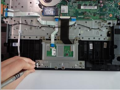
• Unscrew the seven 6mm Phillips screws located around the trackpad.
