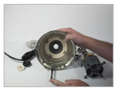
Once motor is pulled out, unscrew the 8 mm screw for the green wire from the base of the blender.
