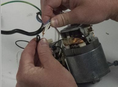
Separate the zip-tie holding the wires to the motor.
