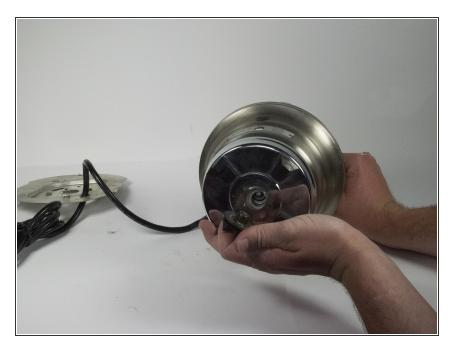
Once the coupling mechanism has been loosened all the way, gently pull it off the top of the blender.
