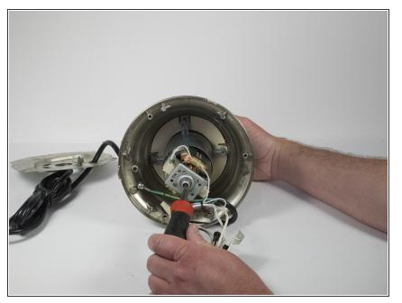
• Place the screwdriver in the head of the middle flat-head screw.
