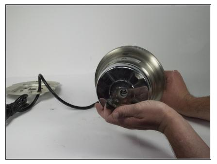
• Once the coupling mechanism has been loosened all the way, gently pull it off the top of the blender.
