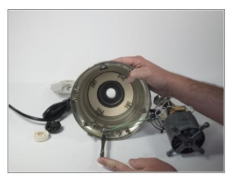
Once motor is pulled out, unscrew the 8 mm screw for the green wire from the base of the blender.
