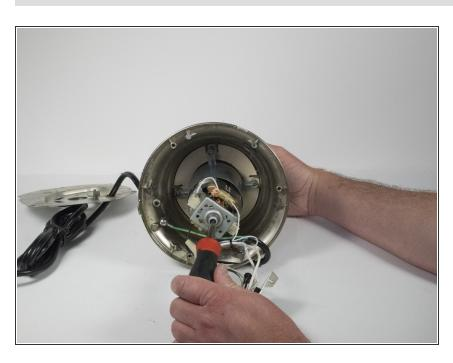
Place the screwdriver in the head of the middle flat-head screw.
