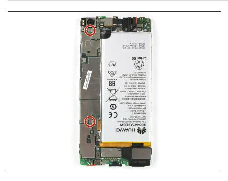
Remove the two Phillips #00 screws that secure the front camera and display/battery connector brackets
