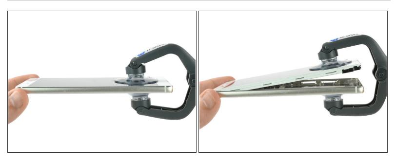
Use an iSclack or a suction handle to separate the display unit from the rear panel.
