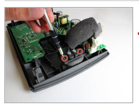
Use a #2 Phillips screwdriver to remove the two 15mm screws from either side of the charging port.
