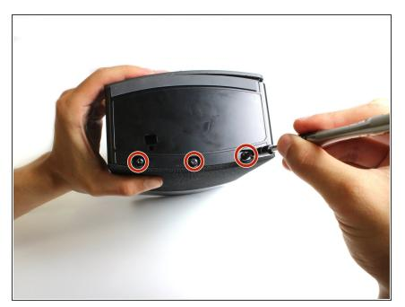
Use a #2 Phillips screwdriver to remove each of the three 20mm screws on the bottom front edge of the speaker.
