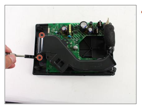
Use a #0 Phillips screwdriver to remove each of the two 11mm screws attached to the bass port.
