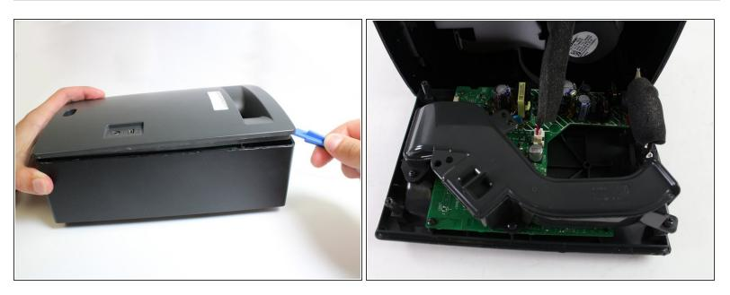
• Use force with an iFixit Plastic Opening Tool to pry the back panel up from the speaker frame.
