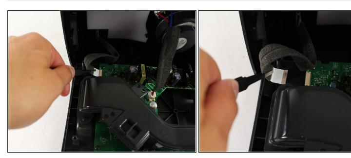
Use ESD Safe Tweezers (Blunt Nose) to pull out the wire ribbon at the end of the motherboard.
