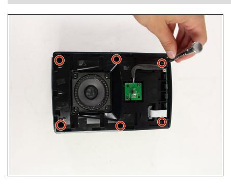
Use a #2 Phillips screwdriver to remove each of the six 20mm screws located underneath the front panel.
