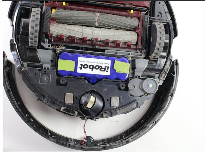
**⚠ Be careful when removing the bumper from the Roomba to prevent damage to the sensor wires. Remove slowly!**
