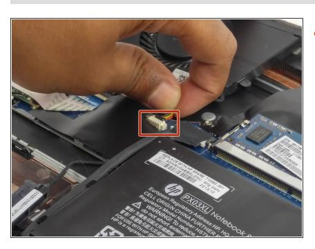
Grab the fan power connector by the wires and pull directly away from port until the cable is disconnected.
