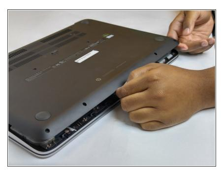
Finally, use both hands to lift up and take off the back plate of the computer.
