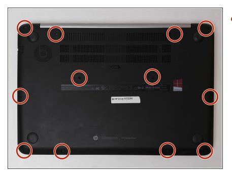
There are 12 phillips head screws which need to be unscrewed before removing the backplate of the laptop.
