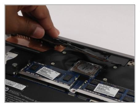
• Lift up the heat sink by the strip of metal connecting it to the exhaust vent, and pull it away from the motherboard.
