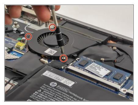
• Use your screwdriver to remove the three screws connecting the fan to the motherboard.
