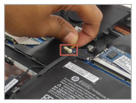
• Grab the fan power connector by the wires and pull directly away from port until the cable is disconnected.
