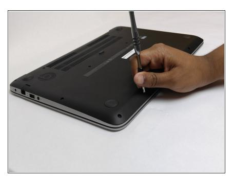
• Next, use a size PH1 Philips head screw driver to remove the screws.
