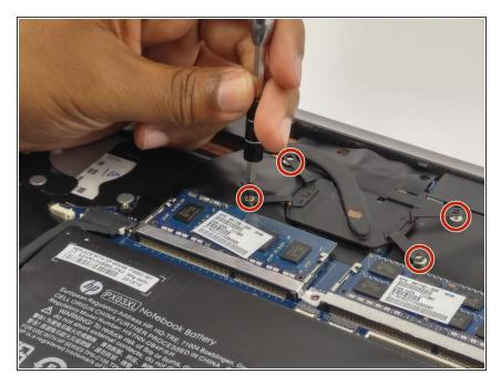
• Unscrew all four of the screws connecting the heat sink to the CPU.
