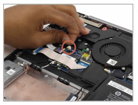
• There is a power cord connecting the CMOS battery to the motherboard. Disconnect this cord by gently pulling it up, towards the edge of the device.
