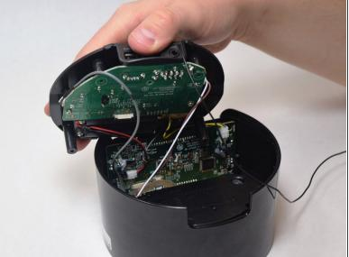
Grip the top of the iBT230 by placing your thumb on the back portion, where the USB port is located. Pull up, and you should notice various different colored wires, connected to the Main Motherboard.
