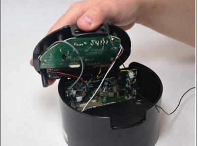
• Grip the top of the iBT230 by placing your thumb on the back of the iBT230, where the USB port is located. Pull up, and you should notice different colored wires connected to the Main Motherboard.
