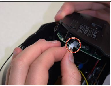
Unplug the connectors from all sides of the iBT230, and unplug the wire that is connected to the screen.
