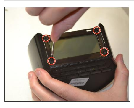
Unscrew the four 5.5 mm Phillips #00 face panel screws from the front screen.
