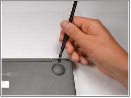
Using a sharp tool, remove the six adhesives from the bottom of your laptop to expose the screwheads underneath. Two of the pads are small and four are larger.
