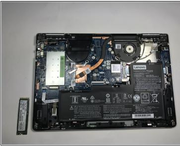
• Use your fingers to lift up the SSD and pull away from the socket removing it from the laptop.
