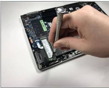
• Use a Phillips #00 screwdriver to remove the 3mm screw on the SSD.
