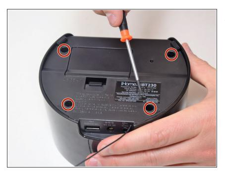
Remove the four 5.5 mm Phillips Head #00 screws from the bottom palate of the iBT230.
