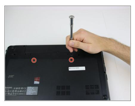
Using a size 00 Phillips Head screwdriver, remove the two M2.5x4 screws connecting the removable plate to the frame of the computer.
