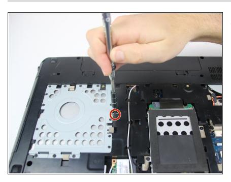
Remove the M2.5x6 screw that fastens the optical drive to the laptop.
