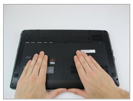
Using both hands, slide the plate off of the back of the laptop.
