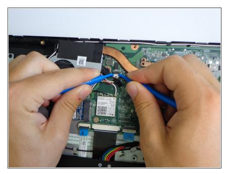
Disconnect the fan from the motherboard by pulling down on the wire connector with two iFixit Opening Tools.
