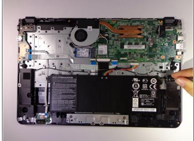
Unscrew the 4mm Phillips #1 screw located at the top right of battery.
