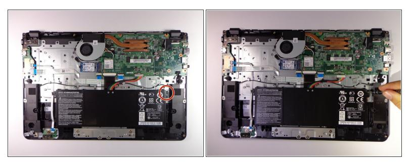
Unscrew the 4mm Phillips #1 screw located at the top right of battery.
