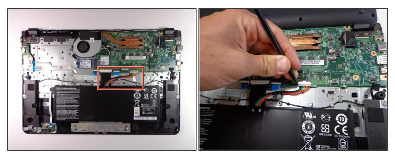
• Using a spudger, carefully unplug the rainbow wires connected to the top of the battery.
