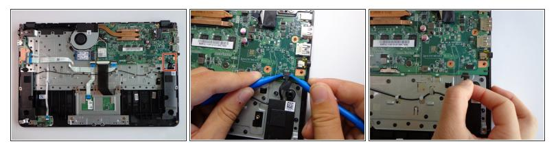
Disconnect the black wires where the speakers are connected to the motherboard by pulling down on both sides with two iFixit Opening Tools.
