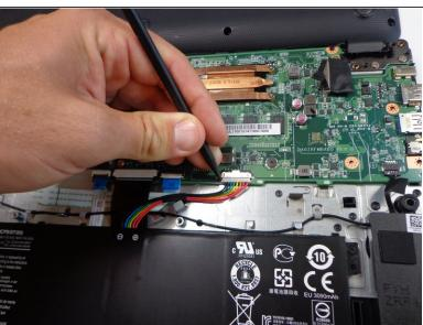
Using a spudger, carefully unplug the rainbow wires connected to the top of the battery.
