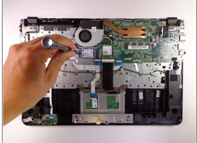
Remove the screw at the left of the drive.
