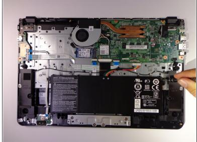
Unscrew the 4mm Phillips #1 screw located at the top right of battery.
