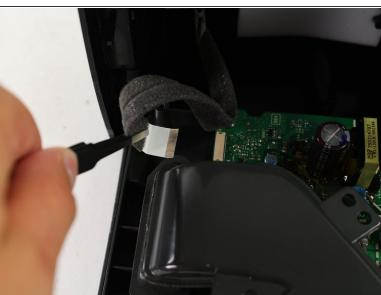
Use ESD Safe Tweezers (Blunt Nose) to pull out the wire ribbon at the end of the motherboard.
