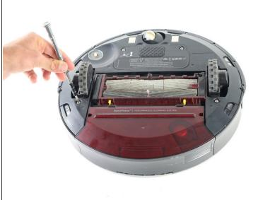
Use the Phillips #00 screwdriver to remove the four 3.5mm screws that hold down the battery panel and rear panel.
