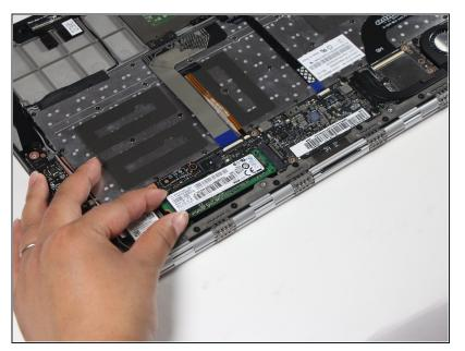
Gently lift and wiggle the SSD side to side to remove it from the laptop chassis.
