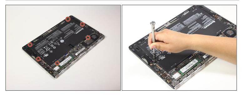
• Remove the six #0 3.8mm Phillips screws from the battery.
