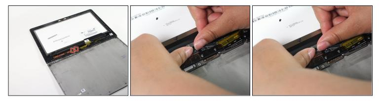
• Disconnect the two monitor connectors with the tips of your fingers.
