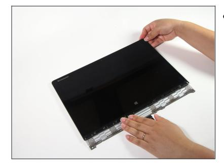
Slowly go around the perimeter of the screen with your fingers to loosen all the tabs holding down the monitor.
