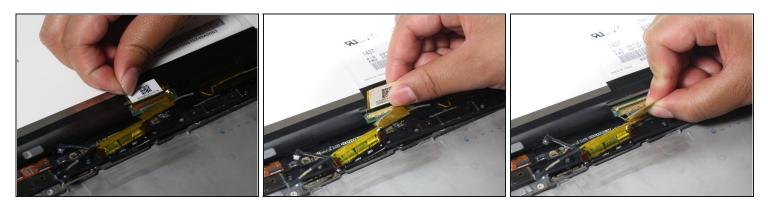
• Remove the flat flex cable by first lifting the hinge then pulling the hinge away from the connector.
