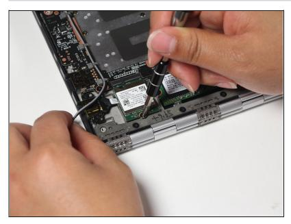
• Remove the one #0 2.9mm Phillips screw from the base of the wifi card.
