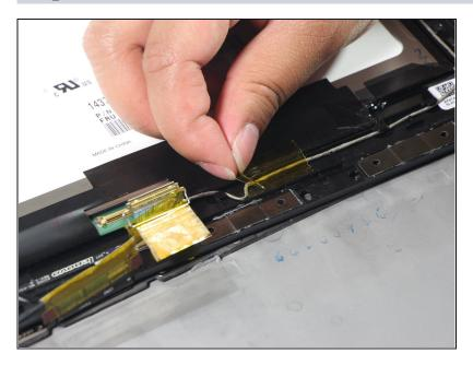
• Peel off the tape holding down the webcam cable.
