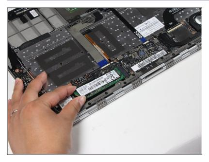
• Gently lift and wiggle the SSD side to side to remove it from the laptop chassis.
