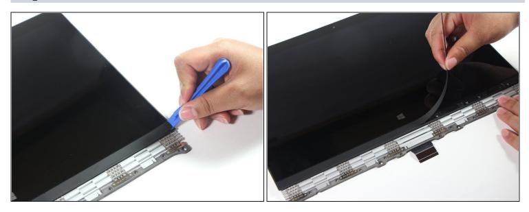
$\triangle$  The screw cover is held down with adhesive and is very fragile.
