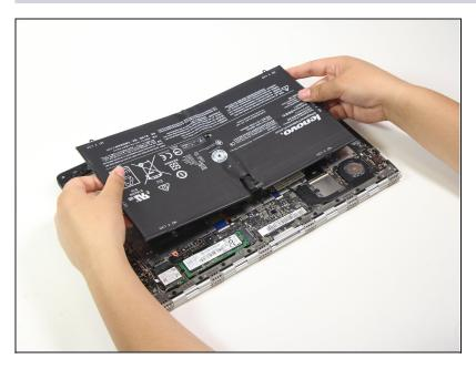
• Gently lift the battery out of the laptop chassis.
