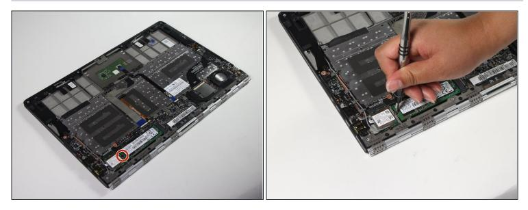
• Remove the one #0 2.9mm Phillips screw from the SSD.
