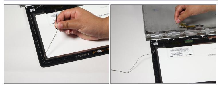
• Carefully unroute the webcam connector from the plastic tabs holding it down.
