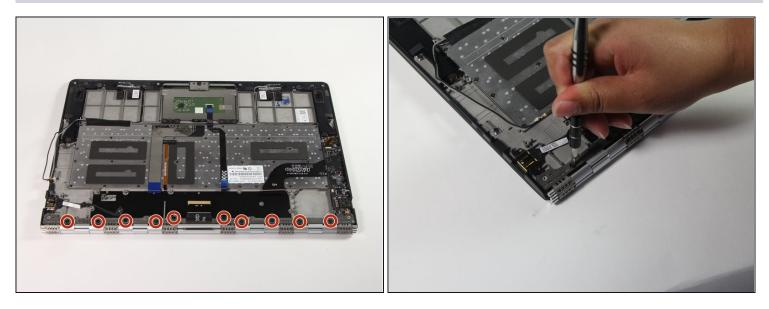
• Remove the ten #0 3.7mm Phillips screws holding down the monitor assembly.
