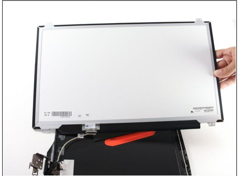
**!** When lifting, be sure to not strain the wires on the left side of the photo, as that could lead to a malfunction in the wires.
