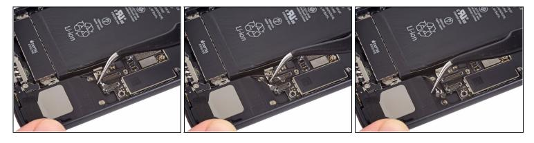
• Use <u>tweezers</u> to gently derout the antenna cables from the metal bracket on the logic board.
