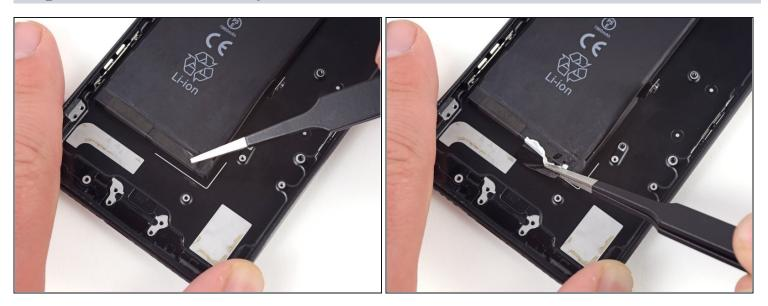
• Use a pair of <u>tweezers</u> with blunt tips to peel back one of the adhesive strips on the lower edge of the battery.
