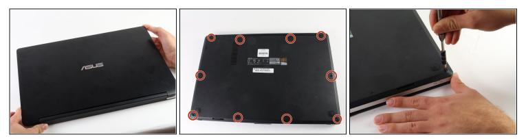
• Remove the ten 10 mm Phillips #0 screws found on the computer's back case.
