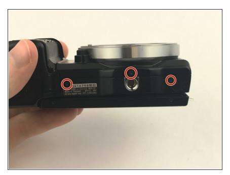
Remove the 3.5 mm bottom screws.
