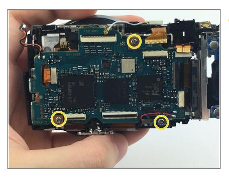
Remove the 4 mm screws securing the motherboard to the frame.
