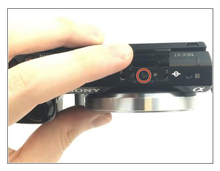
Remove the 3.5 mm top flash-mount screw.
