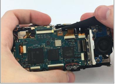
• Using the tweezers, disconnect the metal lead at the top of the motherboard by pulling up.
