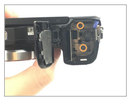
Remove the 4mm screws at the back of the battery compartment.
