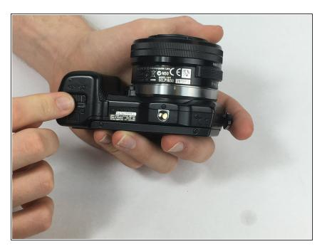
Open the battery compartment by sliding the lock to the right.
