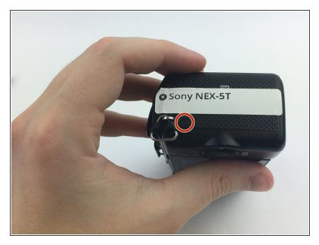
Remove the 3.5 mm exterior-side screw.
