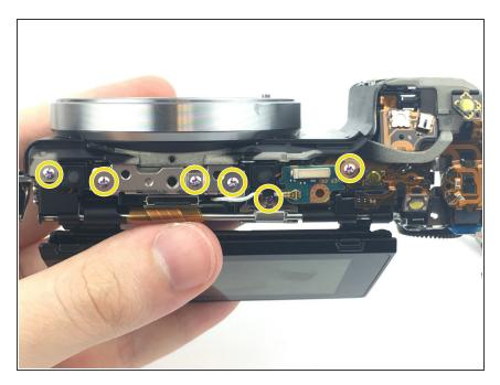
Remove the 2.25 mm screws from the top.
