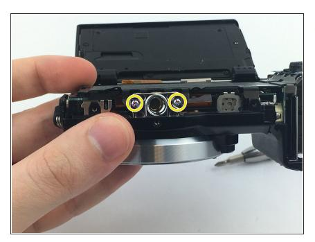
Remove the 2.25 mm tripod mount screws.
