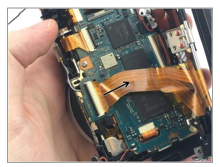
Disconnect the connection between the motherboard and LCD screen by pulling out the connector in the direction of the arrow.
