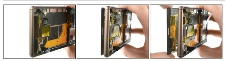
• To fully remove the display off your phone, you need to thread the display flex cable through the gap of the mid frame in the bottom end of your phone.
