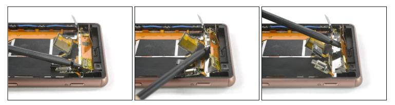
• Use a spudger to gently slide beneath the display flex cable and lift it up.
