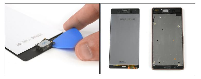
• If you didn't manage to keep the earpiece in its place while removing the display you have to remove it now.
