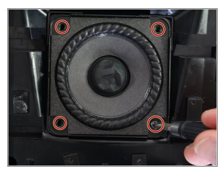
Use a #2 Phillips screwdriver to remove each of the four 15mm screws holding the speaker in place.
