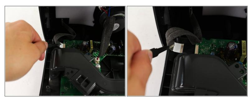
Use ESD Safe Tweezers (Blunt Nose) to pull out the wire ribbon at the end of the motherboard.
