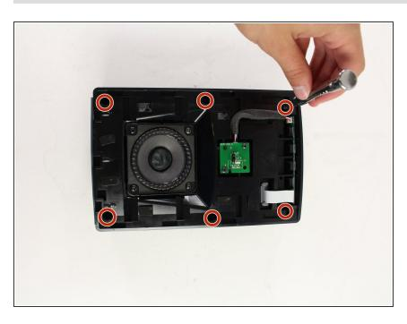
Use a #2 Phillips screwdriver to remove each of the six 20mm screws located underneath the front panel.
