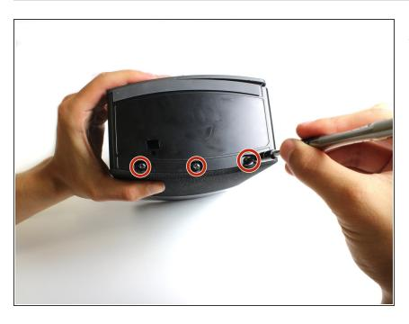
Use a #2 Phillips screwdriver to remove each of the three 20mm screws on the bottom front edge of the speaker.
