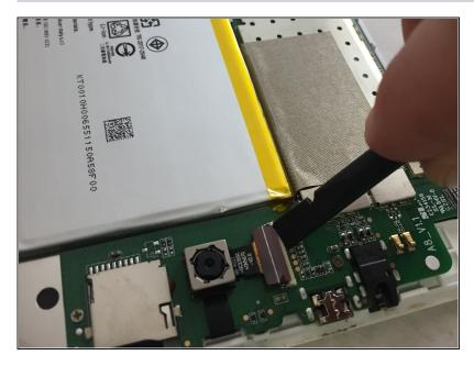
To remove the ZIF connector on the rear camera, gently use the flat end of your spudger to lift it up and free the rear camera.
