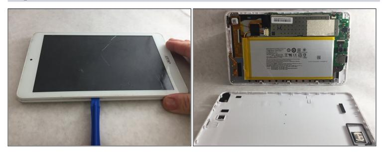
• The first step to replacing the rear camera on your Acer tablet is to remove the Back Panel. To do that, use your iFixit opening tool to pry open the device in the small crevice. Do this gently in order not to crack the screen on your tablet.
