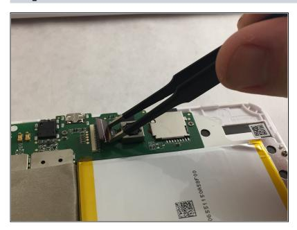
In order to gently remove the camera, grab the precision tweezers and carefully pull out the connector to remove the camera.
