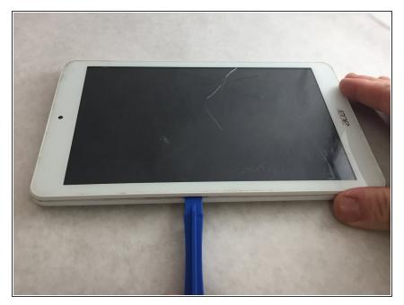
• Use an opening tool to pry open the small crevice in your tablet. Be sure to do this as gently as possible as to not crack the screen of your device.
