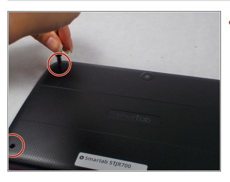
Unscrew all four corner screws using the PH000 screwdriver head found in the iFixit kit.
