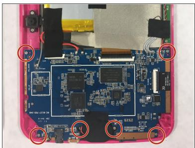
Unscrew all the labeled screws using the PH000 screwdriver head.
