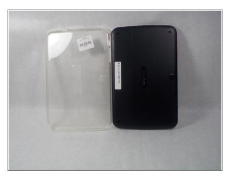
Power off the device by holding down the lock button. Remove the case from the tablet and place it face down.
