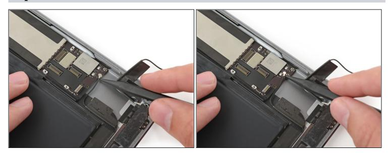
• Insert a spudger under the left antenna cable, the connector farthest from the edge of the iPad. Lift upward to disconnect the antenna cable connector.
