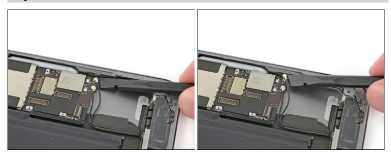
• Insert a spudger under the right antenna cable closest to the edge of the iPad and lift upward to disconnect the antenna cable connector.
