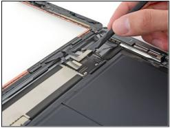
• Use a the flat end of a spudger or a fingernail to carefully pop the two digitizer cable connectors straight up from their sockets.
