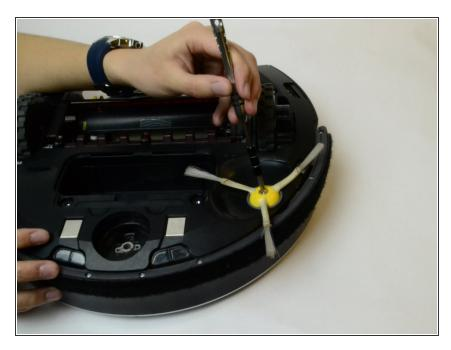
Start by locating the yellow side brush on the underside of the iRobot Roomba 860 near the front of the device.
