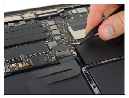
• Remove the trackpad cable connector bracket.
