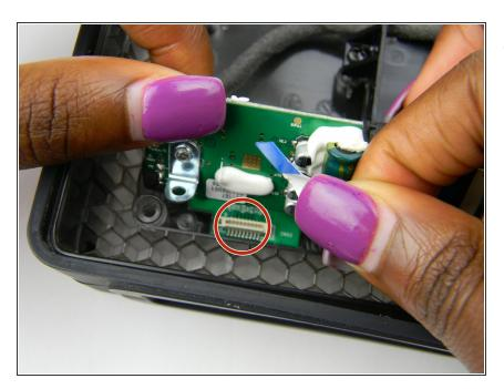
Pull out the cable that is attached to a port under the motherboard.
