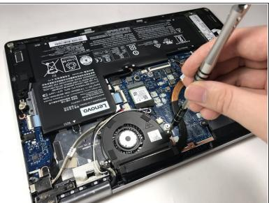
Unscrew the the two 4mm Phillips #00 screws holding the fan in place.
