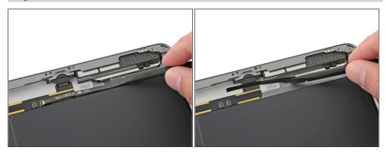
• Gently fold the left speaker ribbon cable up so that it will clear the battery when you slide the speaker enclosure out.
