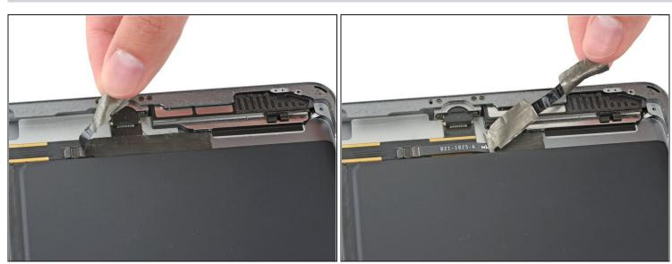
• Remove the tape covering the left speaker cable connector.
