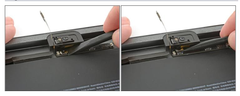
• Use the flat end of a spudger to disconnect the microphone cable connector from the logic board.
