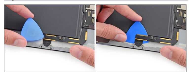
• Finally, slide the opening pick between the battery and the Lightning connector itself to separate the last of the adhesive underneath the cable.
