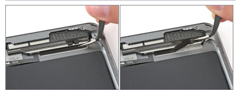
• Remove the tape holding the speaker to the rear case.
