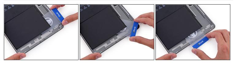
• Slide the card around the lower right corner of the battery.
