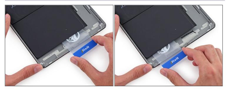
• Slide the plastic card to the lower left corner of the battery.
