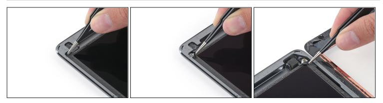
• Remove any tape obscuring the LCD screws.
