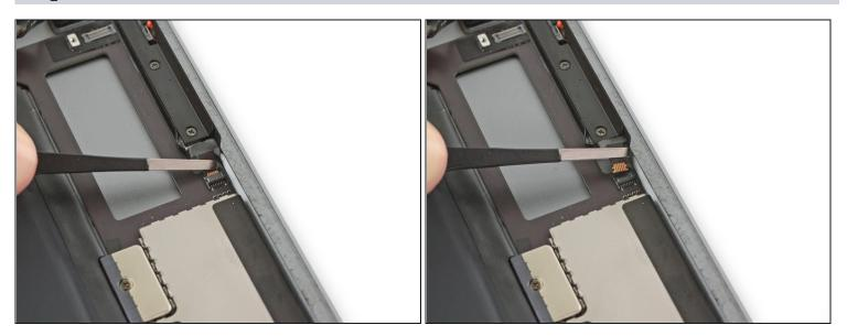
• Slide the upper button assembly cable straight out of its ZIF connector.
