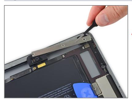
• Remove the upper component cable bracket.
