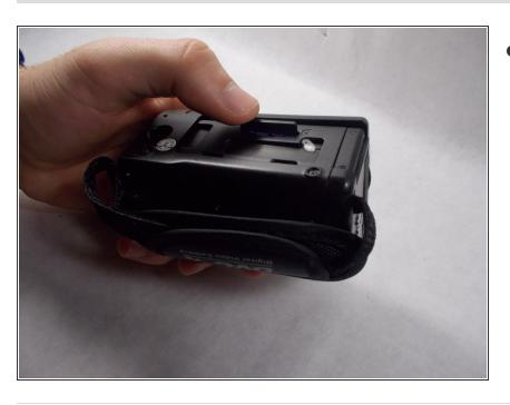
Press down and release pressure quickly on the SD card and remove it out of its socket.
