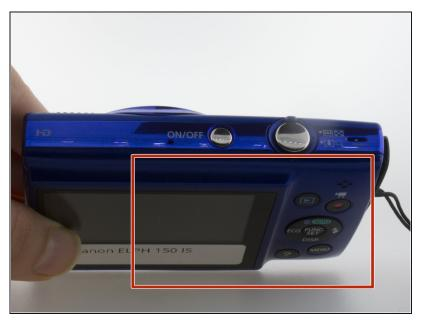
Locate the back plate of the camera (contains the LCD screen and menu buttons).
