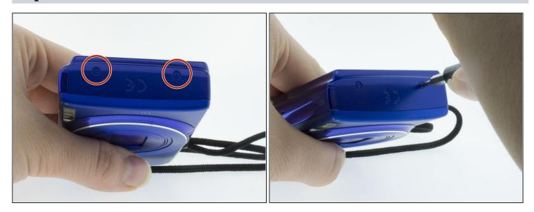
• Use a Phillips #00 screwdriver to remove the final 2 screws from the blue side panel.
