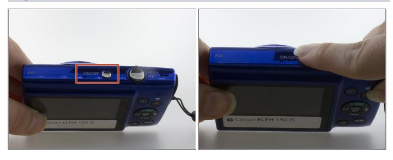
• Locate the ON/Off button on the top of the camera and hold it down until the screen and all lights on the camera go dark.
