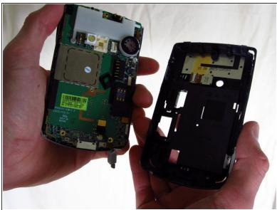
Unplug the sensor wire that connects the two halves of the case before pulling the two halves apart. Not doing so will damage the sensor wire.
