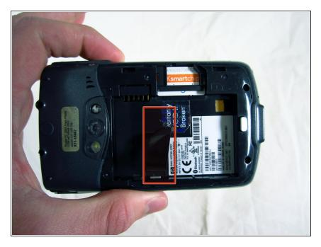
Remove the battery by pulling up on the black tab.
