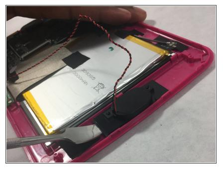
• Use the metal spudger to remove the speaker from the front panel of the tablet.
