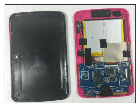
Using a plastic opening tool or metal spudger, begin to gently pry the rear case down and away from the display.Slowly wiggle the tool up and down to pry open the tablet.Once the rear case is fully removed place it to the side.
