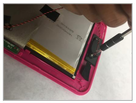
Remove the 2 screws holding the speaker to the front panel. Use a PH000 screwdriver from iFixit kit.
