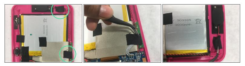
• Using tweezers carefully remove tape that is holding the black and red intertwined cables to the motherboard. Place tape to the side as is will be needed for reassembly.
