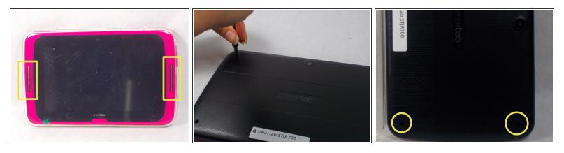
Power off device. Place it face down. Unscrew the 4 perimeter screws, using a PH000 screwdriver from iFixit kit
