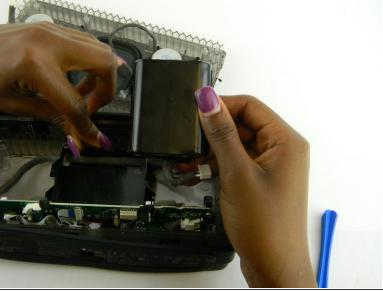
After disconnecting the power supply connector, pull the battery out of its case.
