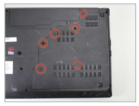
Using a #0 Phillips screwdriver, remove the six 9mm panel screws from the bottom of the device.
