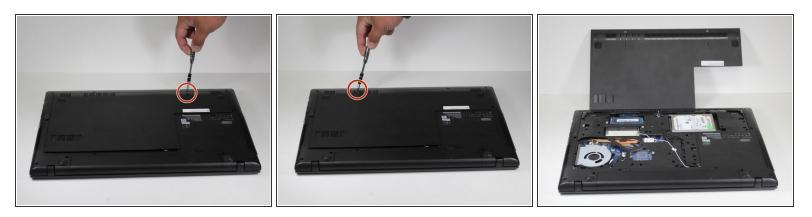
Locate a Phillips head screwdriver. Use the screwdriver to remove the 2 screws found on the backside of the Lenovo G70-80. Once both of these screws are removed you will be able to remove the back of the laptop.
