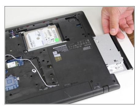
Once all of the hardware in the previous steps is removed, you will be able to pull the CD drive directly out of the laptop.
