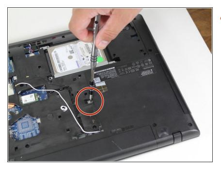
Remove the screw to the left of the CD Drive.
