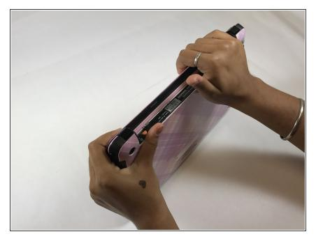
• Remove the battery from the device.
